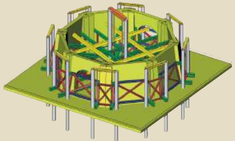
Modelling the windmill base and the lifting jack installation arrangement inside and outside the structure.
