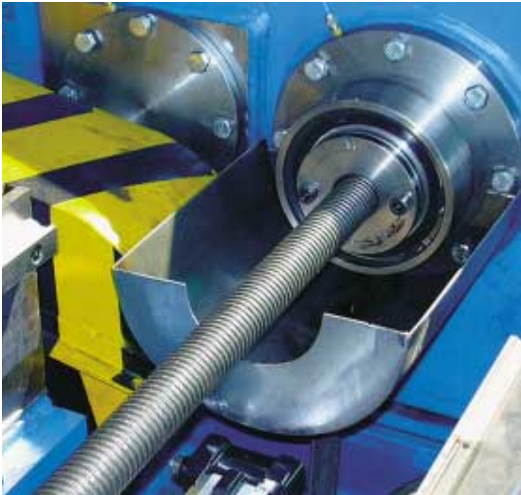
Fabrication benches are used for continuous threading of the Freyssibar bar
